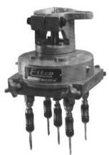
Model 102-5T also utilizes the existing thru drive with center spindle and four (4) eccentric spindles. Spindle coverage options are the same as for 102-5D. The 3/8" serrated spindles each have tapping capacity of 1/4 - 20 cutting taps
