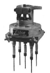
Model 102-5D utilizes the existing thru drive with center spindle and four (4) eccentric spindles. With this unique design spindle coverage can provide: (a) two separate 2 spindle patterns from 31/32 minimum to 3 31/32 maximum, (b) three equally spaced holes from 1" minimum to 2.5 maximum, (c) four equally spaced holes on a 2" minimum bolt circle to 5" maximum bolt circle.
